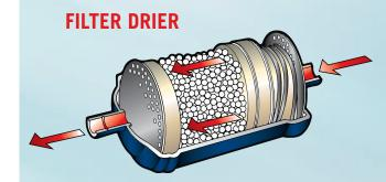
Napoleon air conditioners are built to include the highest quality filter drier in the industry. A filter drier is an extremely beneficial component to your system. Working to remove unwanted acids, dirt, particle debris and other contaminants from the refrigerant, the filter drier extends the life of your air conditioning system.
